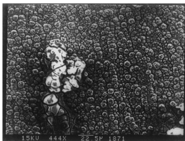
Fig. 5. SEM image of a Ni electrode following a 2 h electrolysis in a 2:1 \text{AlCl}_3 :BTMAC at a constant current density of 5.1 \times 10^{-5} \text{ A cm}^{-2} .
