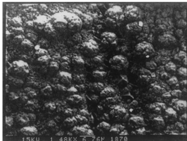
Fig. 8. SEM image of a Ni electrode following a 2 h electrolysis in a 2:1 \text{AlCl}_3 :BTMAC liquid containing 0.03 \text{ mol kg}^{-1} \text{ BTMA}_2 \text{ PtCl}_6 at a constant potential of -0.6 \text{ V} .
